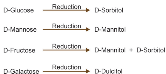
Figure 2.9: Reduction of sugar to form alcohol
